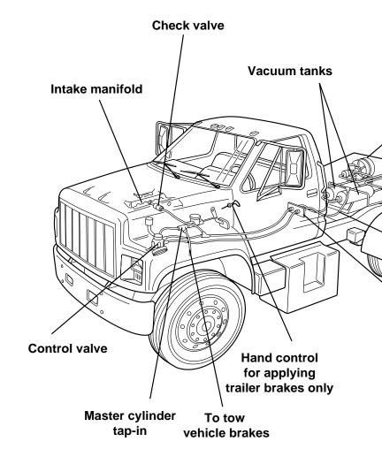
Vacuum / Hydraulic braking system
