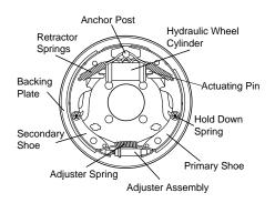
shoe. The secondary shoe is forced onto the anchor pin and from this point, the secondary and primary shoes attempt to 'wrap around'. In essence, the brake has utilized frictional force to help the applying force on both shoes.
