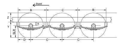
The articulation of this suspension occurs when the spring becomes loaded and consequently lengthens. The double pivot action of the shackle links accommodates this articulation and allows the system to move freely.
